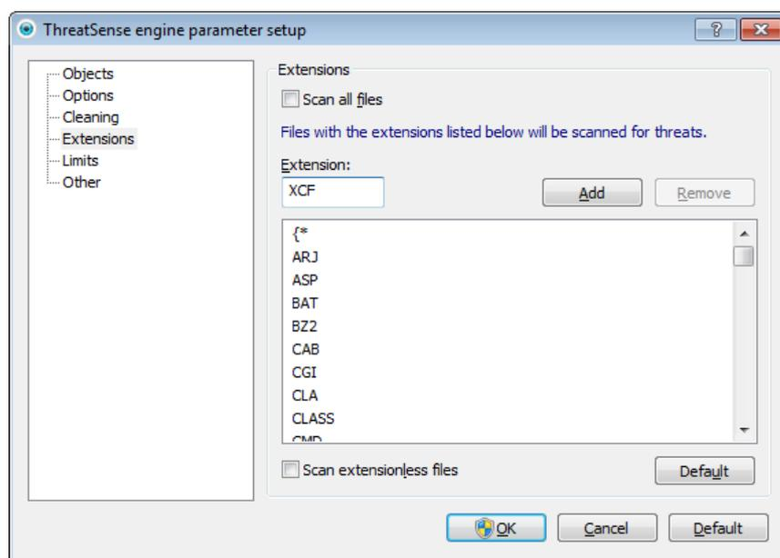
By default, all files are scanned regardless of their extension. Any extension can be added to the list of files excluded from scanning. If the **Scan all files** option is deselected, the list changes to show all currently scanned file extensions.
