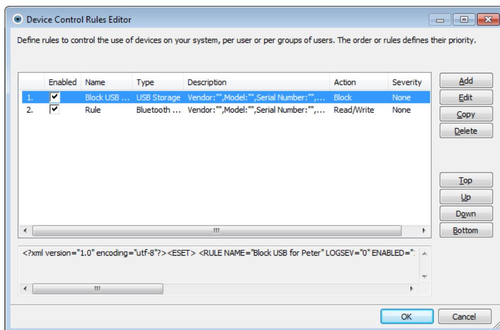
Particular devices can be allowed or blocked per user or user group and based on additional device parameters that can be specified in the rule configuration. The list of rules contains several descriptions of a rule such as name, type of external device, action to perform after connecting an external device to your computer and log severity.
