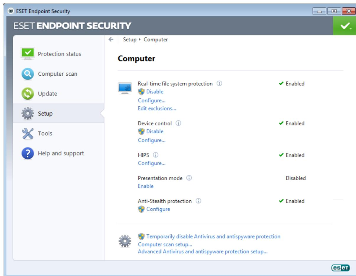
**Temporarily disable Antivirus and antispyware protection** – Disables all antivirus and antispyware protection modules. **Temporary disable protection** dialog box with **Time interval** drop-down menu will display. A **Time interval** drop-down menu represents the period of time that the protection will be disabled. Click **OK** to confirm.
