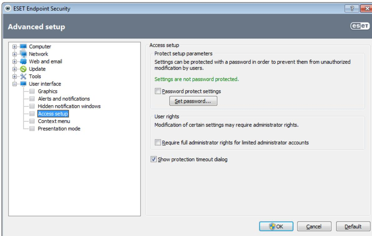
Enter a password into the **New password** and **Confirm new password** fields and click **OK**. This password will be required for any future modifications to ESET Endpoint Security settings.
