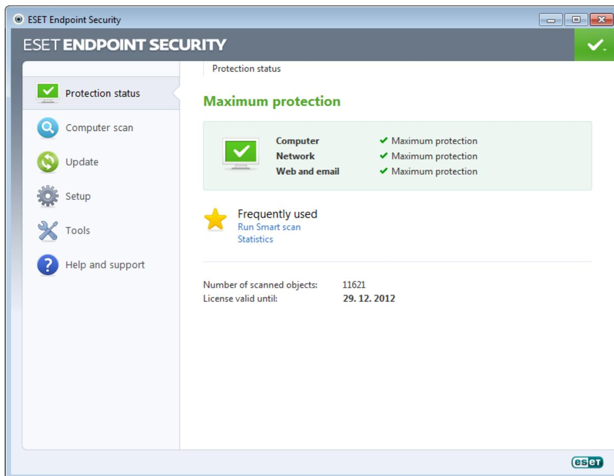
The **Protection status** screen informs you about the security and current protection level of your computer. The green **Maximum protection** status indicates that maximum protection is ensured.
